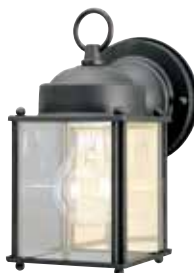
66972 Wall Fixture Textured Black Finish Clear Glass Panels Height: 8.25" Width: 4.50" Extends: 5.75" Height from Center of Outlet Box: 3.00" Back Plate: D: 4.50" Use (1) Medium (E26) Base Lamp, 100 Watt Maximum
