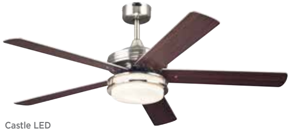
72091 Castle LED 52 in. Brushed Nickel Finish Reversible Blades (Weathered Maple/Beech) Opal Frosted Glass Includes (2) Medium (E26) Base, 8 Watt T7 LED Lamps (WL Lamp #33199) Pull Chains Included
