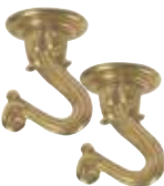
70450 1 1/2" Swag Hook Kit Polished Brass Finish Includes: • 2 Hooks • 2 Spring Toggle Wings • 2 Running Thread Studs: #10-24 x 2 7/8" • 2 Wood Screws: #10 x 1 1/4" • 30 lb. Load Rating
