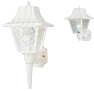
66946 Polycarbonate Wall Fixture with Removable Tail White Finish Clear Textured Acrylic Height with Tail: 17.00" Height without Tail: 13.00" Square: 8.00" Extends: 8.50" Height from Center of Outlet Box: 10.75" Back Plate: H: 4.63" W: 4.63" Use (1) Medium (E26) Base Lamp, 60 Watt Maximum
