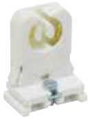
*22454 Medium BiPin Turn Type Lamp Holder Low Profile Size No. 18/20 Gauge Panel Mount, Captive Mount and Screw 660 Watts Max., 600 Volts Non Shunted
