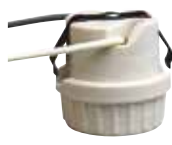
*22212 Porcelain Snap-In Socket Medium Base 6" Wire Leads Fits 1½" Hole 18 Gauge, 125° Leads 660 Watts Max., 250 Volts Height - 1¾"
