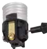
*22504 3-Way Turn-Knob Socket Medium Base 250 Watts Max. 250 Volts Height - 1¼"
