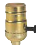
70412 - 3-Way 70413 - On/Off 70421 - 2 Circuit Turn-Knob Socket Brass Finish Medium Base Tapped ½-IP 250 Watts Max., 250 Volts
