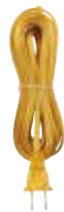
70103 15' Cord Set Gold Polarized Plug 18-2 SPT-2, 105" Wire Free ends are Split, Stripped and Tipped
