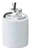
*22370 70425 Porcelain Fixture Socket Medium Base 10" Wire Leads, Height - 2½" ½-IP Hickey 18 Gauge, 105° Leads 660 Watts Max., 250 Volts
