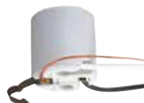
*22372 Porcelain Snap-In Socket Medium Base 9" Wire Leads Fits ¾" x ¼" Hole 18 Gauge, 105° Leads 660 Watts Max., 250 Volts Height - 2"
