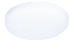
70058 Blank-Up Kit White Finish Diameter - 5" Holes Spaced, 2 3/4" Apart Includes: • 1 Canopy, 1 Crossbar, 2 Mounting Screws, 2 Cap Nuts • 50 lb. Load Rating
