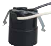
*22213 1 ½" Snap-in Socket 6" Wire Leads Medium Base Fits 1¼" Hole 18 Gauge 105° Leads 660 Watts Max., 250 Volts Height - 1½"
