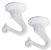
70770 1 1/2" Swag Hook Kit White Finish Includes: • 2 Hooks • 2 Spring Toggle Wings • 2 Running Thread Studs: #10-24 x 2 7/8" • 2 Wood Screws: #10 x 1 1/4" • 30 lb. Load Rating
