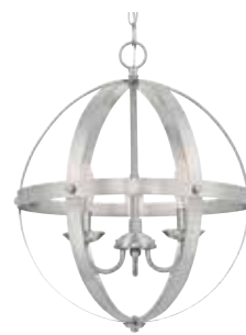
63419 Stella Mira 3 Light Chandelier Brushed Nickel Finish Height: 17.25" Diameter: 15.00" Chain: 36" Cord: 60" Use (3) Candelabra (E12) Base Lamps, 40 Watt Maximum
