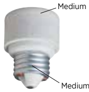
*22150 Porcelain Socket Extender Medium Base 660 Watts Max., 250 Volts Extension - 1/4" Overall Length - 2 1/4"
