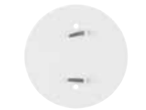
†29453 70064 White Outlet Concealer Holes Spaced 2 3/4" Apart Diameter - 4 3/4" Mounts on 3" or 4" Outlet Box Includes: • 2 8-32 x 3/4" White Head Screws †Polybagged Bulk Items
