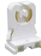
*22453 Medium BiPin Lamp Holder Low Profile Size 660 Watts Max., 600 Volts T8/T12 Non Shunted
